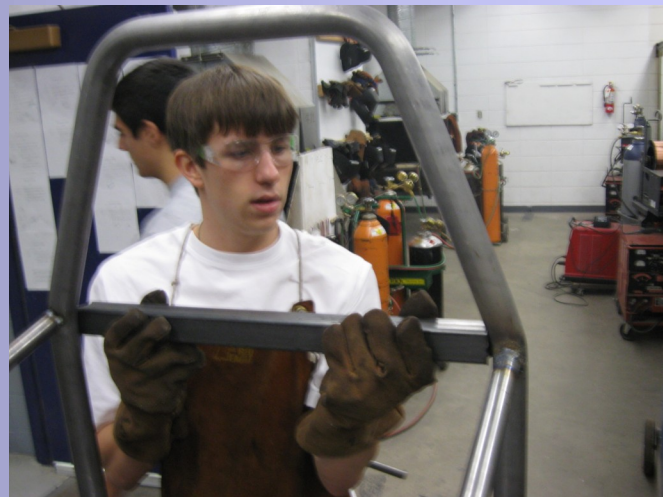
Nick cutting a piece of the tubing so the ends will butt against the curved tubing properly.
