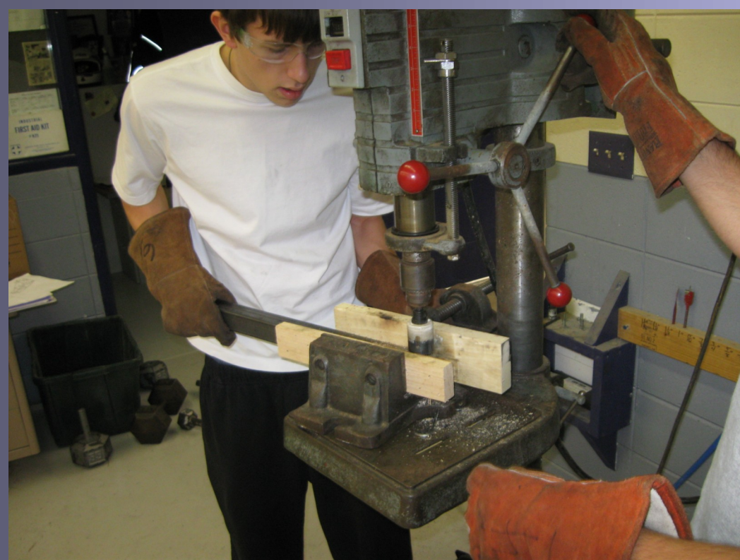
Nick cutting a piece of the tubing so the ends will butt against the curved tubing properly.
