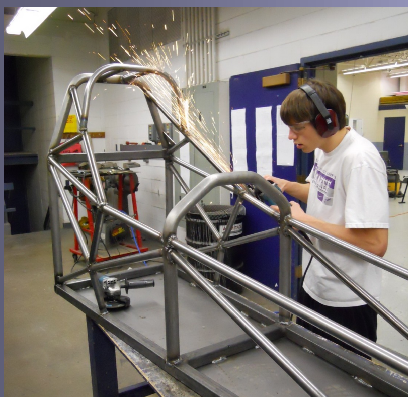
Nick grinding off the excess material on the welds.
